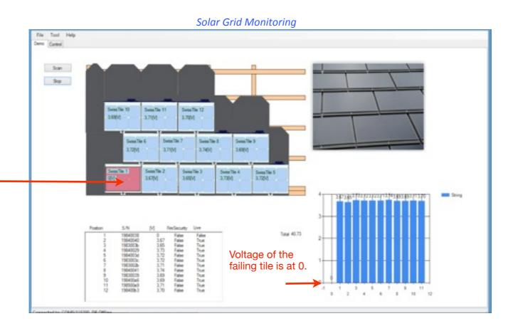
In case of malfunction, the failing tile is instantaneously identified and display in red on the screen. You can see immediately which tiles is not functioning.
