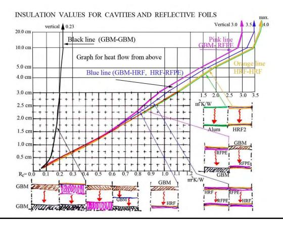
The calculations are based on reflectivity (r) and emissivity ( $\epsilon$ ) of materials:  $r + R_C + \epsilon = 1$  in which the  $R_C$  is the insulation value of the foil itself (very little).
